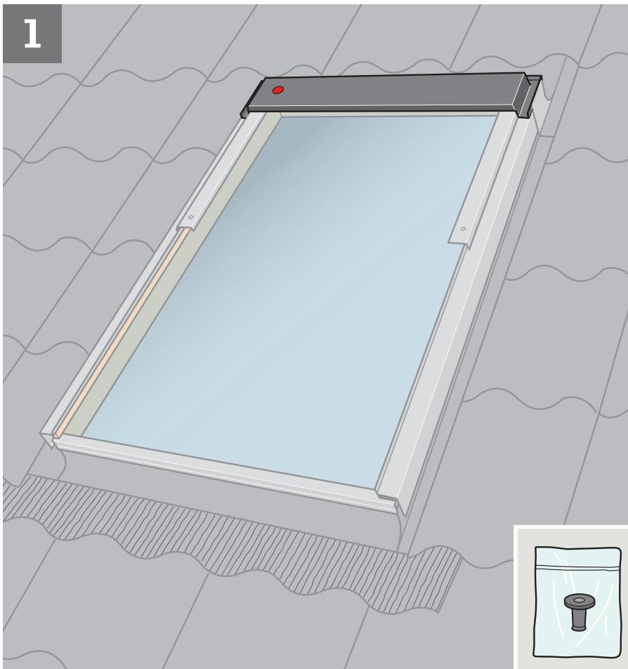
**ENGLISH:** If the window has been fitted with a connection box, remove this temporarily **a**. Drill hole **b** or **c** and fit rubber grommet **d**. Pull grommet through from the inside **e**.
